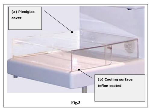
Equipped with Plexiglas cover **(Fig.3 a)** to maintain constant temperature and avoid the formation of ice and the creation of condensation.on the cooling surface.
