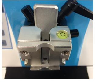
The orientation of the samples is possible in a simple and precise; if the red lights are visible, then the guidance plan is in zero position. The steel clamp is equipped with a device to "clamp" for quick change of the sample and sample holder fixed tilt.
