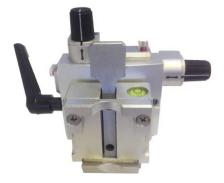
The steel clamp is equipped with a device to "clamp" for quick change of the sample and sample holder fixed tilt.
