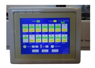
Using the control panel, you can view and modify the operating parameters, such as processing programs, the temperature of the compartments paraffin door. Also it allows for daily and weekly programming on and off.
