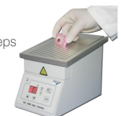
Histo Trimmer to remove excess paraffin from biocassettes
