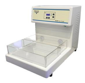
TEC 2900-2 Cryo Console is designed to allow rapid cooling of paraffin blocks.
